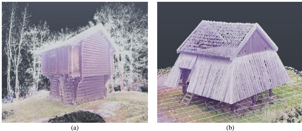
Figure 8: Raw point cloud data for (a) Heierstad Loft, (b) Fadum Storehouse
