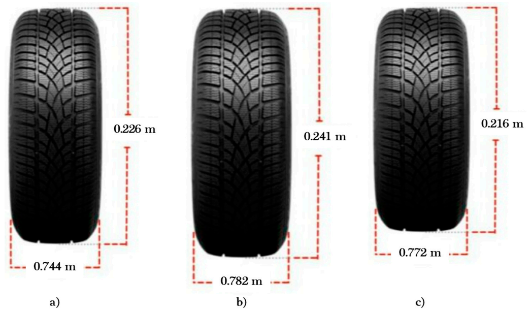
Figure 5. Dimensions of Tires Used: (a) 225/75R16, (b) 235/80R16, (c) 215/85R16.
