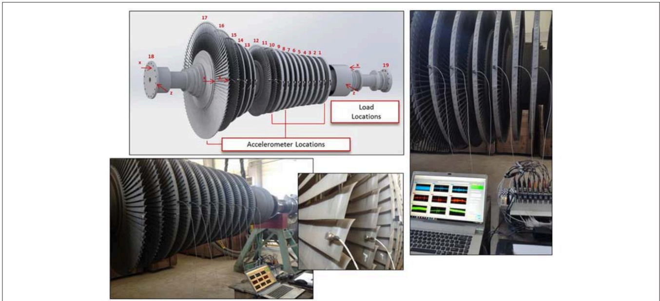
FIGURE 7 | Experimental set-up of the intermediate pressure turbine.
